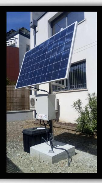
Fully autonomous microseismic cabinet designed for painless operation
